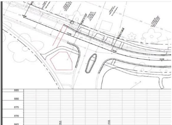
2. <u>Spring Harbor Park Bioswale (South)</u> – At AHC's request, the City explored adding additional stormwater features on public assets. This allowed the City, after discussion with Parks, to add a 50 foot bioswale at park. There is space to push the sidewalk back to accommodate this feature. Faith suggested making it longer and connect to apron drain. Emphasized vegetated swales and filters over infiltration.
